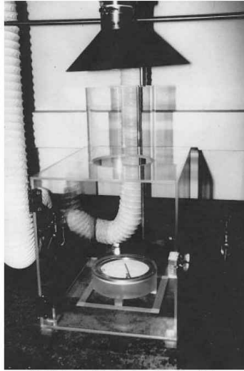
FIG. 1 Photograph of Test Chamber and Filter Paper Holder
